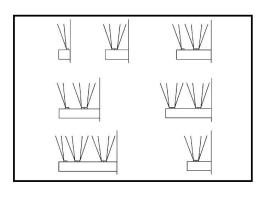
Correctly spaced installations for various surface widths plus projections extending exposed edge
