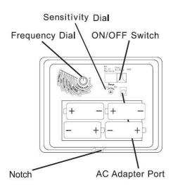
Batteries Install four "C" batteries as shown on the unit. Snap the cover back into place.
