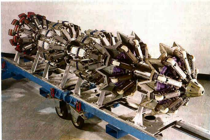
5. Where no pig has gone before. GE's new SmartScan tool can scan pipelines that are impassable to pigs due to valve restrictions, multiple pipeline diameters, or too many sharp bends. Courtesy: GE Power
